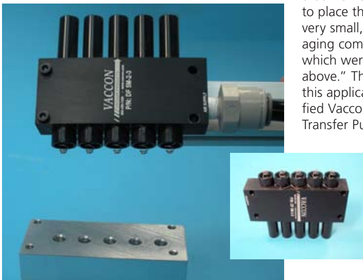
Above and inset, right. A modified Vaccon DF Series Material Transfer pump holding five coiled springs. A robotic arm positions the pump over the individual spring compartments in the packaging, allowing the springs to drop into individual packaging cells and avoid tangling.
