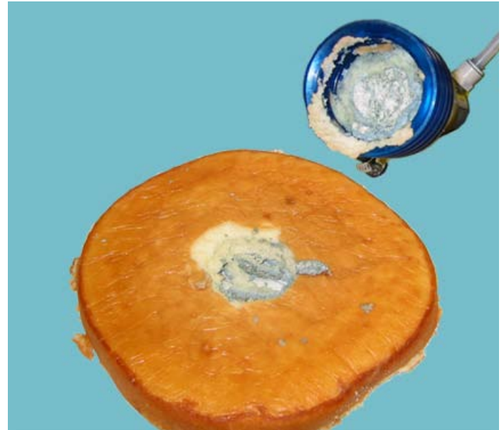
Conventional vacuum and vacuum cup technology damages delicate, "crumbly" products like cake.
