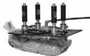
Picking and placing packaged rolls, CDF 375H-ST6BX EOAT handles flexible, uneven objects.
