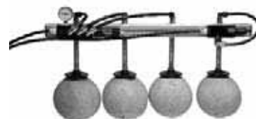
VP80-200H-MP and VP20-100H EOAT handle melons in fruit packing plant.
