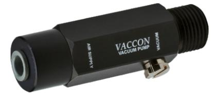
1. Install in-line vacuum pump to your mounting hardware, end-of-arm-tool, extrusion, etc.. The optional panel mount nut can be used to secure the pump to a panel. The exhaust port has a 5/8-18 UNF male thread. The panel through hole should be at least 7/8" [21 mm].
