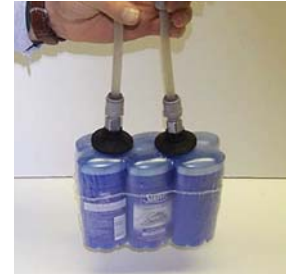
VP10 with bellows cups – pick and place deodorant packages for packaging application.
