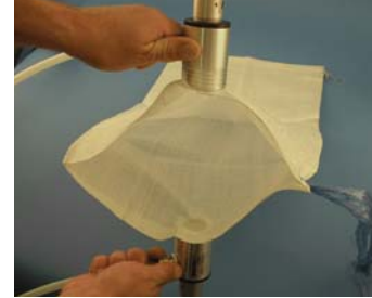
Two CDF pumps handle cheesecloth fabric bag – bag opening and closing application.
