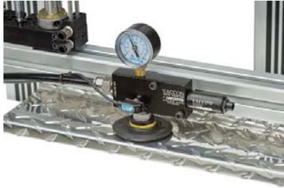
VP20 pump with bellows cup picks up diamond tread plates – stacking application.
