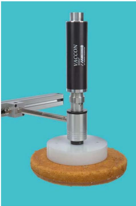
*To accommodate the physical characteristics of cake, a round, rigid cup with mesh screening and composed of Ultra High Molecular Weight (UHMW) plastic was developed. This allows a greater surface area for suction, creating a vacuum head able to spread the vacuum tension over the entire top surface area of the cake without marring or dimpling.*
