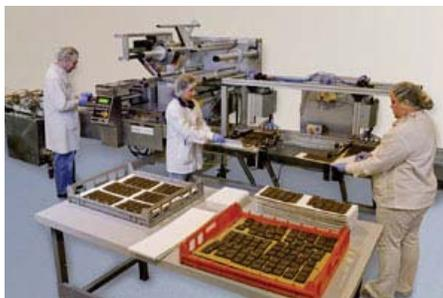
**Operators no longer have to place miniBARS one-at-a-time between the spacing lugs on the wrapper infeed chain. The new pick-and-place system is faster and less labor-intensive.**
