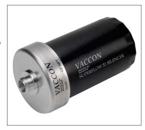
The FA-51 silencer is made up of two components: a threaded adapter and a replaceable filter element. The replaceable element has a large area inside to absorb sound and debris, creating a safer, quieter work environment. The FA-51 silencers are available in 3 thread sizes: 1/4" NPT, 3/8" NPT, and 1/2" NPT. The exhaust port of the pneumatic device determines the size of the silencer. Maximum operating pressure is 150 PSIG.
