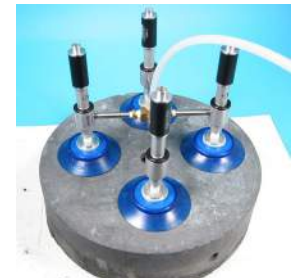
VDF pumps with flat cleated cups handle 42 lb graphite spacer for nuclear industry.
